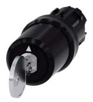
Key-operated switch BKS, 22 mm, round, plastic, lock number S1, with 2 keys, 3 switch positions I>O<II, momentary contact on the left, latching on the right, actuating angle  $2x45^{\circ}$ , 10:30h/12h/13:30h, Key removal O
