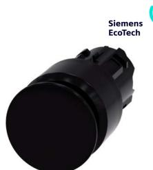
Mushroom pushbutton, 22 mm, round, plastic, black, 30 mm, latching, pull-to-unlatch mechanism, Z=50-unit packaging
