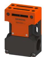
safety position switch with separate actuator plastic, short enclosure, 3x(M20x1.5), lateral and face-end operation, slow-action contacts 1 NC pull-out force 30 N, supplied without actuator
