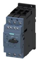
Circuit breaker size S2 for motor protection, CLASS 10 A-release 35...45 A N-release 650 A screw terminal Standard switching capacity with transverse auxiliary switches 1 NO+1 NC
