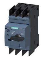
Circuit breaker size S00 for motor protection, CLASS 10 A-release 0.45...0.63 A N-release 8.2 A ring cable lug connection Standard switching capacity
