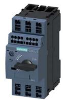
Circuit breaker size S00 for motor protection, CLASS 10 A-release 0.45...0.63 A N-release 8.2 A Spring-type terminal Standard switching capacity with transverse auxiliary switches 1 NO+1 NC
