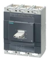
Molded case circuit breaker 3RV1 for starter combination Standard switching capacity Rated current In = 630 A electronic release Short-circuit protection adjustable 1-10 x In Icu = 100 kA at 400 V 3-pole, Screw terminal including phase barriers
