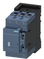
capacitor contactor, AC-6b 100 kVAr, / 400 V, 3-pole, 83-155 V AC/DC, 50/60 Hz, with integrated varistor, auxiliary contacts: 2 NC, screw terminal, size: S3  $\,$
