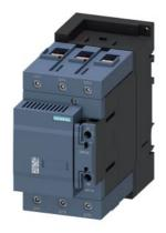
capacitor contactor, AC-6b 100 kVAr, / 400 V, 3-pole, 230 V AC, 50 Hz, auxiliary contacts: 1 NO + 1 NC, screw terminal, size: S3  $\,$
