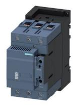
capacitor contactor, AC-6b 100 kVAr, / 400 V, 3-pole, 110 V AC, 50 Hz, auxiliary contacts: 1 NO + 1 NC, screw terminal, size: S3  $\,$
