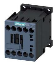
power contactor, AC-3, 16 A, 7.5 kW / 400 V, 4-pole, 220 V DC, main contacts: 2 NO + 2 NC, screw terminal, size: S00  $\,$
