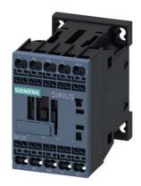
power contactor, AC-3, 12 A, 5.5 kW / 400 V, 4-pole, 48 V DC, with integrated diode, main contacts: 2 NO + 2 NC, spring-loaded terminal, size: S00
