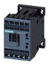
power contactor, AC-3, 12 A, 5.5 kW / 400 V, 4-pole, 48 V DC, main contacts: 2 NO + 2 NC, spring-loaded terminal, size: S00  $\,$
