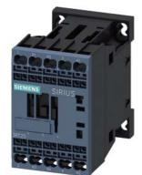
power contactor, AC-3, 9 A, 4 kW / 400 V, 4-pole, 110 V AC, 50/60 Hz, main contacts: 2 NO + 2 NC, spring-loaded terminal, size: S00
