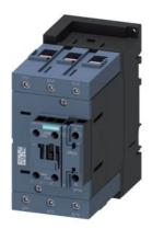
contactor AC-1, 140 A, 690 V / 40 °C, 3-pole, 400 V AC, 50 Hz, auxiliary contacts: 1 NO + 1 NC, main circuit: box terminal, control and auxiliary circuit: screw terminal, size: S3  $\,$
