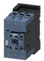
contactor AC-1, 140 A, 690 V / 40 °C, 3-pole, 220 V AC, 50 Hz / 240 V, 60 Hz, auxiliary contacts: 1 NO + 1 NC, main circuit: box terminal, control and auxiliary circuit: screw terminal, size: S3
