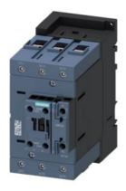
contactor AC-1, 140 A, 690 V / 40 °C, 3-pole, 110 V AC, 50 Hz / 120 V, 60 Hz, auxiliary contacts: 1 NO + 1 NC, main circuit: box terminal, control and auxiliary circuit: screw terminal, size: S3
