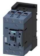
contactor AC-1, 140 A, 690 V / 40  $^\circ$ C, 3-pole, 24 V AC, 50/60 Hz, auxiliary contacts: 1 NO + 1 NC, main circuit: box terminal, control and auxiliary circuit: screw terminal, size: S3
