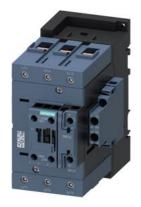
power contactor, AC-3e/AC-3, 95 A, 45 kW / 400 V, 3-pole, 230 V AC, 50/60 Hz, auxiliary contacts: 2 NO + 2 NC, screw terminal, size: S3, lateral auxiliary switch
