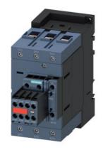
power contactor, AC-3e/AC-3, 80 A, 37 kW / 400 V, 3-pole, 24 V DC, 0.8-1.2\* Us, with integrated varistor, auxiliary contacts: 1 NO + 1 NC, screw terminal, size: S3, suitable for PLC outputs, captive auxiliary switch
