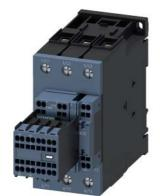
traction contactor, AC-3e/AC-3, 80 A, 37 kW / 400 V, 3-pole, 110 V DC, 0.7-1.25\* Us, electronic drive, with integrated varistor, auxiliary contacts: 2 NO + 2 NC, main circuit: screw terminal, control and auxiliary circuit: spring-loaded terminal, size: S2, removable auxiliary switch
