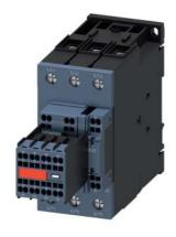
power contactor, AC-3e/AC-3, 80 A, 37 kW / 400 V, 3-pole, 110 V AC, 50 Hz / 120 V, 60 Hz, auxiliary contacts: 2 NO + 2 NC, main circuit: screw terminal, control and auxiliary circuit: spring-loaded terminal, size: S2, captive auxiliary switch
