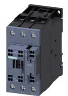
power contactor, AC-3e/AC-3, 65 A, 30 kW / 400 V, 3-pole, 230 V AC, 50/60 Hz, auxiliary contacts: 1 NO + 1 NC, main circuit: screw terminal, control and auxiliary circuit: spring-loaded terminal, size: S2
