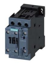
power contactor, AC-3e/AC-3, 25 A, 11 kW / 400 V, 3-pole, 220 V DC, auxiliary contacts: 1 NO + 1 NC, screw terminal, size: S0  $\,$
