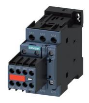
power contactor, AC-3e/AC-3, 25 A, 11 kW / 400 V, 3-pole, 24 V DC, auxiliary contacts: 2 NO + 2 NC, screw terminal, size: S0, captive auxiliary switch, no surge suppressor retrofittable
