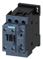
power contactor, AC-3e/AC-3, 25 A, 11 kW / 400 V, 3-pole, 208 V AC, 50/60 Hz, auxiliary contacts: 1 NO + 1 NC, screw terminal, size: S0, upright mounting position
