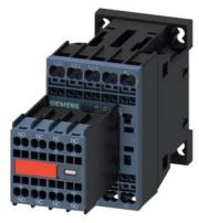
power contactor, AC-3e/AC-3, 12 A, 5.5 kW / 400 V, 3-pole, 24 V DC, with integrated diode, auxiliary contacts: 2 NO + 2 NC, spring-loaded terminal, size: S00, captive auxiliary switch
