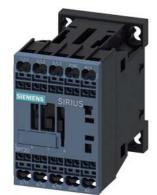
power contactor, AC-3e/AC-3, 12 A, 5.5 kW / 400 V, 3-pole, 24 V DC, with integrated diode, auxiliary contacts: 1 NC, spring-loaded terminal, size: S00
