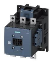
power contactor AC-1 400 A / 690 V / 40  $^{\circ}$ C 3-pole, Uc: 200-220 V AC(50-60 Hz) / DC drive: conventional auxiliary contacts 2 NO + 2 NC main circuit: busbar control and auxiliary circuit: screw terminal
