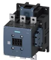
power contactor AC-1 400 A / 690 V / 40  $^\circ$ C 3-pole, Uc: 23-26 V AC(50-60 Hz) / DC drive: conventional auxiliary contacts 2 NO + 2 NC main circuit: busbar control and auxiliary circuit: screw terminal
