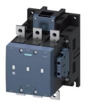
vacuum contactor AC-3e/AC-3 300 A, 160 kW / 400 V, 3-pole, Uc: 380-420 V AC(50-60 Hz) / DC drive: conventional auxiliary contacts 2 NO + 2 NC main circuit: busbar control and auxiliary circuit: screw terminal
