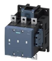
vacuum contactor AC-3e/AC-3 300 A, 160 kW / 400 V, 3-pole, Uc: 200-220 V AC(50-60 Hz) / DC drive: conventional auxiliary contacts 2 NO + 2 NC main circuit: busbar control and auxiliary circuit: screw terminal
