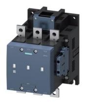
vacuum contactor AC-3e/AC-3 300 A, 160 kW / 400 V, 3-pole, Uc: 42-48 V AC(50-60 Hz) / DC drive: conventional auxiliary contacts 2 NO + 2 NC main circuit: busbar control and auxiliary circuit: screw terminal
