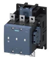
vacuum contactor AC-3e/AC-3 225 A, 110 kW / 400 V, 3-pole, Uc: 200-277 V AC(50-60 Hz) / DC PLC input 24 V DC drive: electronic auxiliary contacts 2 NO + 2 NC main circuit: busbar control and auxiliary circuit: screw terminal
