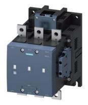
vacuum contactor AC-3e/AC-3 225 A, 110 kW / 400 V, 3-pole, Uc: 21-27.3 V AC(50-60 Hz) / DC PLC input 24 V DC drive: electronic auxiliary contacts 2 NO + 2 NC main circuit: busbar control and auxiliary circuit: screw terminal
