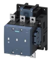
vacuum contactor AC-3e/AC-3 225 A, 110 kW / 400 V, 3-pole, Uc: 380-420 V AC(50-60 Hz) / DC drive: conventional auxiliary contacts 2 NO + 2 NC main circuit: busbar control and auxiliary circuit: screw terminal
