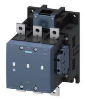
vacuum contactor AC-3e/AC-3 225 A, 110 kW / 400 V, 3-pole, Uc: 240-277 V AC(50-60 Hz) / DC drive: conventional auxiliary contacts 2 NO + 2 NC main circuit: busbar control and auxiliary circuit: screw terminal
