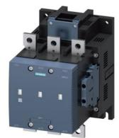
vacuum contactor AC-3e/AC-3 225 A, 110 kW / 400 V, 3-pole, Uc: 23-26 V AC(50-60 Hz) / DC drive: conventional auxiliary contacts 2 NO + 2 NC main circuit: busbar control and auxiliary circuit: screw terminal
