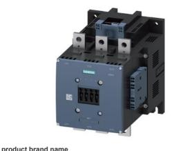
power contactor, AC-3e/AC-3 500 A, 250 kW / 400 V AC (50-60 Hz) / DC Uc: 21-27.3 V PLC input 24 V DC 3-pole, auxiliary contacts 2 NO + 2 NC drive: electronic main circuit: busbar control and auxiliary circuit: spring-loaded terminal
