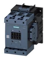
power contactor, AC-3e/AC-3 185 A, 90 kW / 400 V AC (50-60 Hz) / DC Uc: 23-26 V 3-pole, auxiliary contacts 2 NO + 2 NC drive: conventional main circuit: box terminal control and auxiliary circuit: screw terminal
