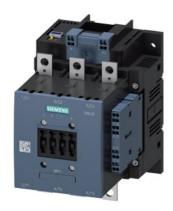
power contactor, AC-3e/AC-3 115 A, 55 kW / 400 V, AC (50-60 Hz) / DC Uc: 96-127 V PLC input 24 V DC 3-pole, auxiliary contacts 2 NO + 2 NC drive: electronic main circuit: busbar control and auxiliary circuit: spring-loaded terminal
