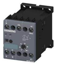
Timing relay, electronic slow-operating 1 change-over contact 24 V AC/DC, 200 to 127 V AC at 50/60 Hz AC 0.05 s to 100 h Overall width 45 mm screw terminal
