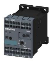
Timing relay, electronic Multifunction, 16 functions 2 change-over contacts 24 to 240 V AC/DC at 50/60 Hz AC 0.05 s to 100 h Overall width 45 mm Spring-type terminal
