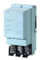
ET 200pro DSE ST DOL starter Standard Mechanical switching Electronic overload protection AC-3, 5.5~kW / 400~V 1.50~A...12.00~A without brake contact Han Q4/2 - Han Q8/0
