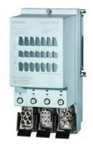
ET 200pro EDSE/DSSE HF electronic DOL starter electronic (soft-) switching Full motor protection consisting of: electronic overload protection + thermistor 400 V 3 AC/0.9 kW 0.15 A...2.00 A Brake contact 400 V AC 4 DI Han Q4/2 - Han Q8/0
