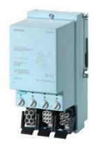
ET 200pro RSE HF Reversing starter High Feature Mechanical switching Electronic overload protection AC-3, 0.9 kW / 400 V 0.15 A...2.00 A Brake contact 400 V AC 4 DI Han Q4/2 - Han Q8/0
