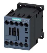
Coupling contactor relay, 3 NO + 1 NC, 24 V DC, 0.7  $\dots$  1.25\* US, with integrated suppressor diode, Size S00, screw terminal suitable for PLC outputs
