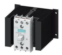
Solid-state contactor 3-phase 3RF2 AC 51 / 40 A / 40  $^{\circ}$ C 48-600 V / 110 V AC 3-phase controlled screw terminal Blocking voltage 1200 V
