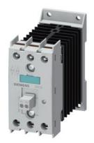
Solid-state contactor 3-phase 3RF2 AC 51 / 20 A / 40  $^{\circ}\text{C}$  48-600 V / 110 V AC 2-phase controlled screw terminal Blocking voltage 1200 V
