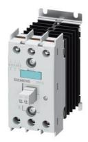
Solid-state contactor 3-phase 3RF2 AC 51 / 10 A / 40  $^{\circ}\text{C}$  48-600 V / 110 V AC 3-phase controlled screw terminal Blocking voltage 1200 V
